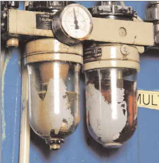
Figure 16. Typically aged units still working on a CNC machine.
